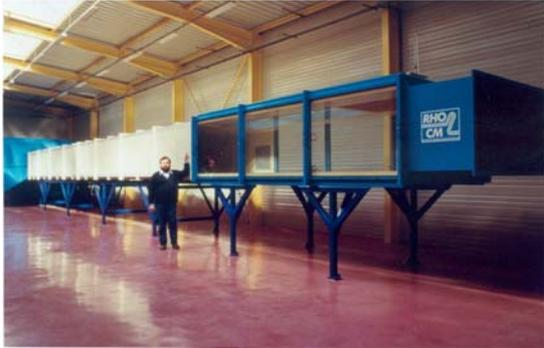
Fig. 1 : LML Boundary Layer Wind Tunnel
