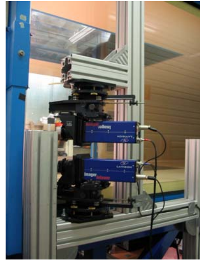
Fig. 4 : Double Stereo PIV set up to record 3C velocity fields in the plane normal to the main flow.
